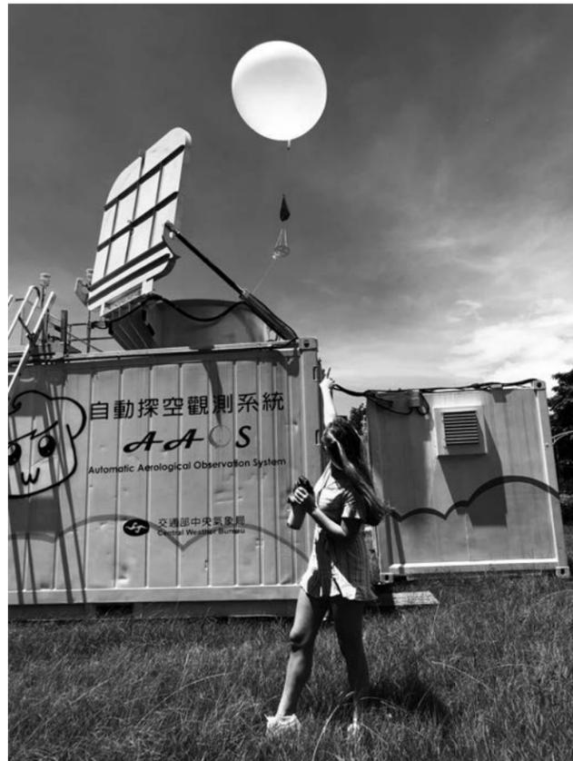
Taiwan's Central Weather Bureau (CWB) Automatic Radiosonde Launcher. Radiosondes launched at 00 UTC, 06 UTC, 12 UTC, and 18 UTC for the PRECIP field campaign. Source: Angelie Nieves Jiménez at Hsinchu, Taiwan (PRECIP 2022)
